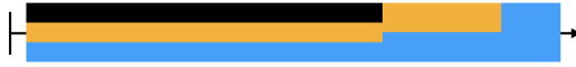
(b) Continuous version of the round-robin order. Instead of scheduling the black job, for example, round-robin for 2 discrete timesteps, we schedule it in parallel with the two other jobs for six timesteps at a rate of \frac{1}{3} .
