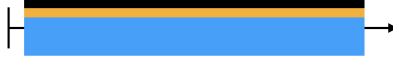
Figure 4: Illustration of preferential round-robin under the following conditions: \lambda = \frac{1}{2} , there are three jobs, and the blue job has the shortest predicted processing time. The black and the yellow jobs are run at a rate of \frac{1-\lambda}{3} = \frac{1}{6} and the blue job is run at a rate of \lambda + \frac{1-\lambda}{3} = \frac{2}{3} .
